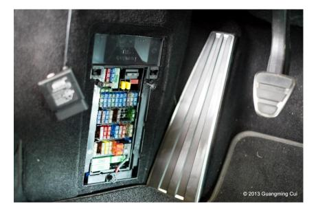
View of the fuse box area (987.2, 981 GT4 similar). The forward end of the kick panel cover has hard Velcro fasteners that pull apart straight out and the rear has plastic pins facing forward at the bottom rear and facing back (into a tang hanging down from the dash) at the top rear. BE CAREFUL removing this panel, but no special tools (or any tools) are required.
