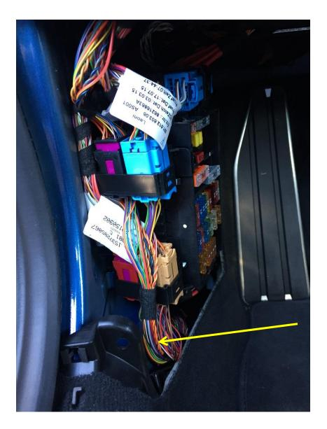
With the panel off, here are the two "gateway" connectors that connect the rear harness to the dash and instrument cluster harnesses.
