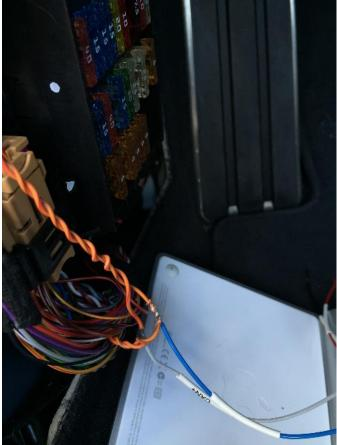
Extract the twisted pair from the bundle. CAREFULLY use an Exacto knife or sharp scissors to cut the black fabric tape binding the loom below the connectors.
